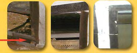
Problem solved! To meet Ed's performance criteria Industrial Energy Products, Inc. developed a tadpole gasket utilizing Silicone impregnated Glastemp fabric over a closed cell neoprene sponge core. The new Glastemp tadpole seals proved to seal the irregular surfaces and have the durability to with stand repeated washings. A door seal that was purchased and installed weekly can now be replaced with a Glastemp seal that can provide years of efficient service.
