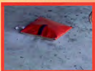
BAG HOLDS EXPLOSIONS AND MINIMIZES SMOKE RELEASE
